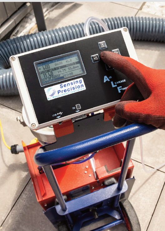
Imperial Ductwork Services are utilising MEP Hire's ALF150 mobile duct leakage testing units at Royal Albert Dock London.
