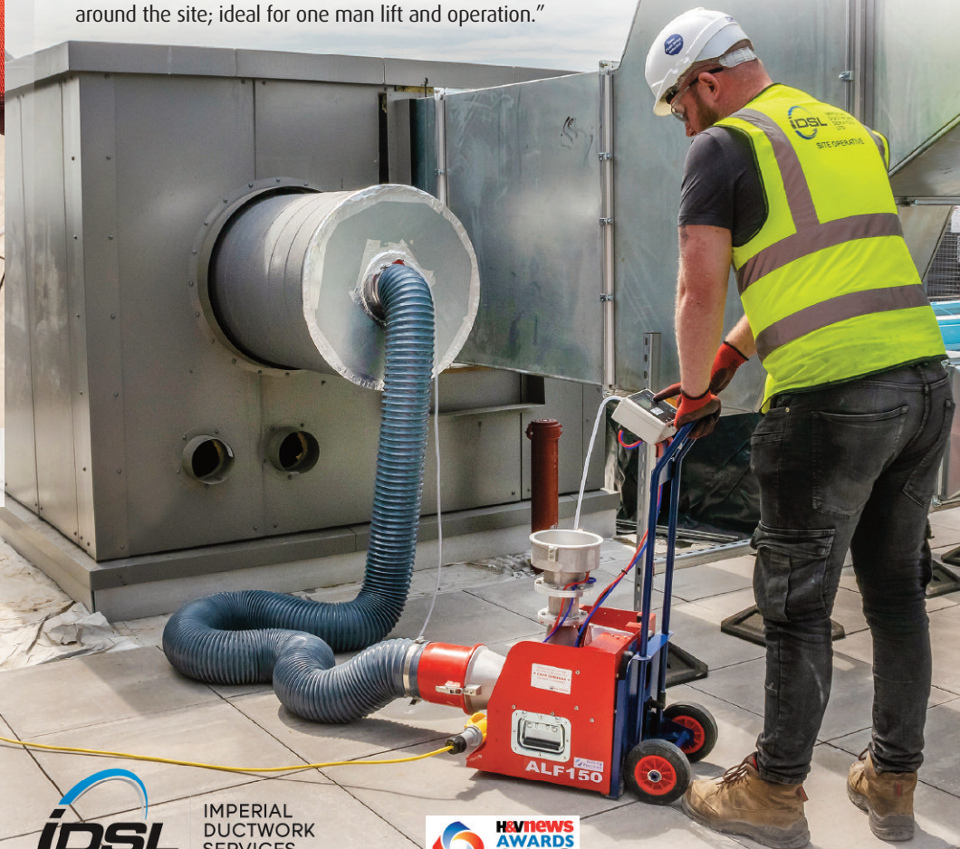
Imperial Ductwork Services are utilising MEP Hire's ALF150 mobile duct leakage testing units at Royal Albert Dock London.
